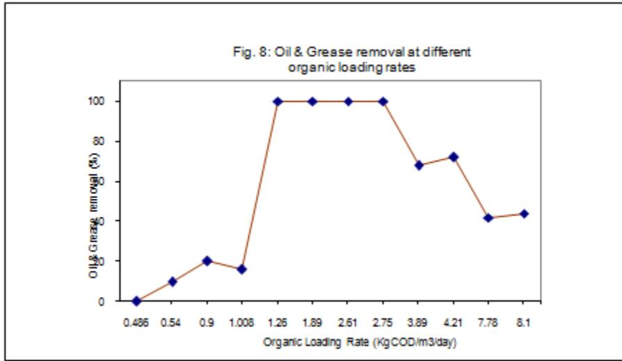
The problem associated with the fat in anaerobic reactors is that the biodegradation of waste waters rich in fat was slower than that of waste waters with a low fat content. Thus the presence of fats in the waste water prevent the periodic production of high concentrations of VFA, which may adversely affect the subsequent processes.
