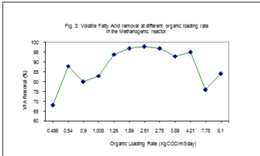
Percent utilization VFA in Phase II was 68% only. However, it could enhance upto 88% because of the high start-up of the reactor. High start-up was made possible by having the seed slurry from a distillery unit which was running successfully. Maximum utilization rate of about 97-98% was achieved in Phase VI but in Phase VII it came down to 76-84% due to recued HRT as already stated Fig. 3.
