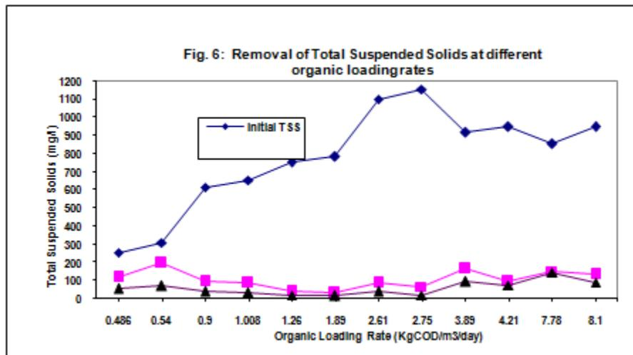
The removal rate was increased with increasing organic load, the substrate utilization rate was also increased with increasing activity of microorganisms. Thus, the reduction rate was increased in the subsequent phases Fig. 6.
