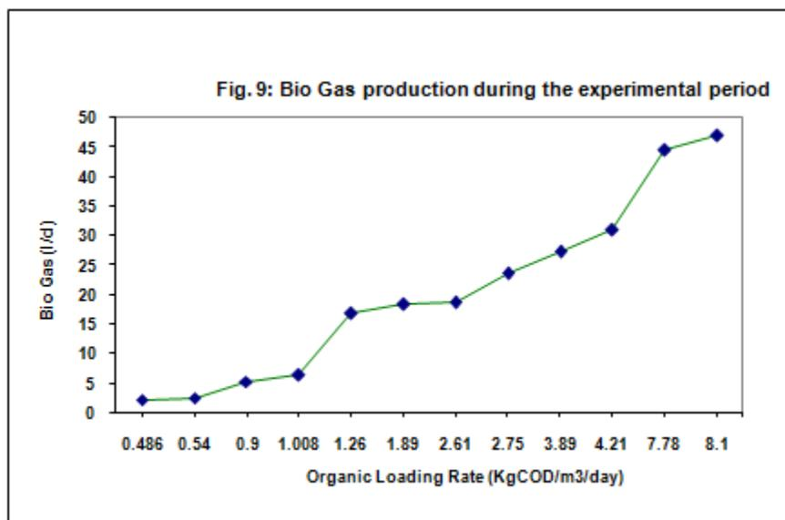
A slight time delay of gas production was observed initially due to the time required for activating the bacteria that converts the biomass into CH<sub>4</sub> and CO<sub>2</sub>. There after the biogas production rate kept on increasing in the subsequent days. The biogas production was not affected even at lowering of HRT, indicating the two phase UASB reactor is more efficient.
