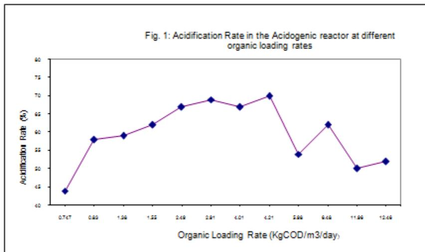
At an HRT of 2 days, the maximum VFA production was recorded in all the phases. The maximum acidification rate was reported in Phase V, the acidification rate was 67-70% at an organic loading rate of 4.01-4.21 kg COD/m<sup>3</sup>/day in the acidogenic phase (Fig. 1). At an HRT of 2 days, the increasing of COD concentrations results in production of more Volatile Fatty Acids and their acidification rate also were high. While reduction of HRT by 1
